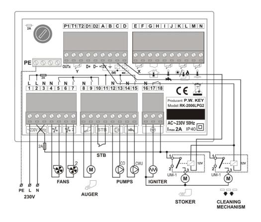
Figure 2. RK-2006LPG2 Controller connection diagram.
