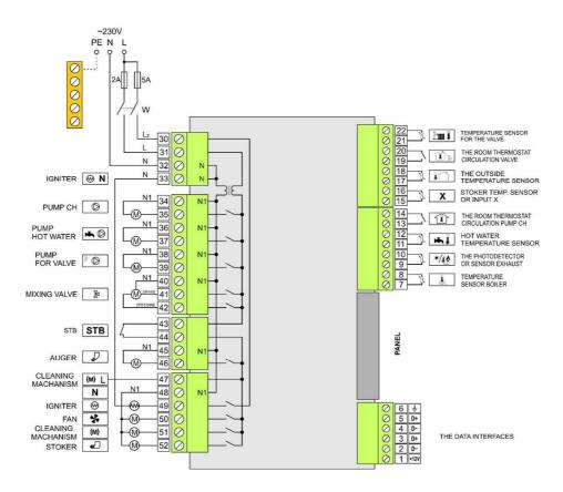
Figure. RK-2006SPGMS Controller connection diagram.
