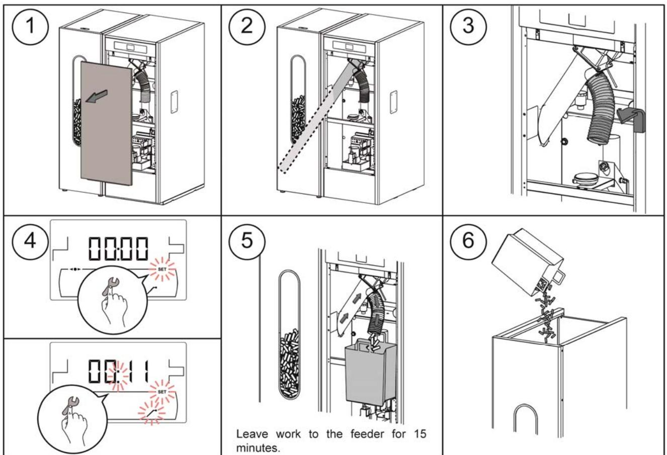
**IMPORTANT:** It is compulsory to fill the feed auger during the commissioning or when the hopper runs out of fuel.
