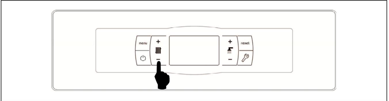
Boiler temperature set point selection is made by the tactile selector shown in the picture. Press "+" and "-" buttons to increase or decrease the set point desired. Few seconds after the desired set point temperature is adjusted the display returns to main position. The range of values for boiler temperature set point is OFF, 65 - 80 °C.
