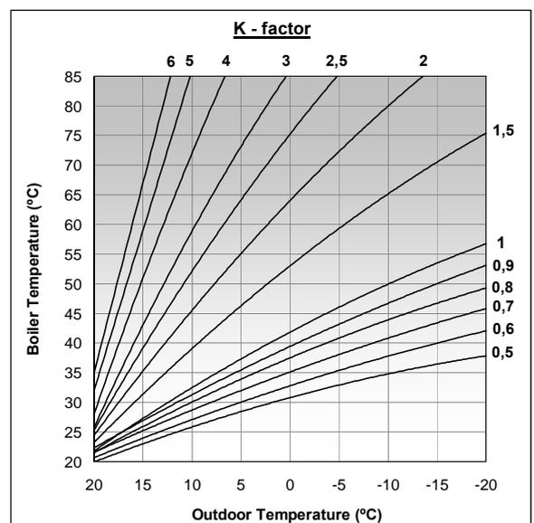
Depending on the type of heating circuit, isolation of the building and position of the outdoor sensor, the optimal K-factor curve could be different. Nevertheless, a general rule could be that for high temperature heating circuits (radiators heating circuit) the K-factor curve should be 1 or higher and for low temperature heating circuits (underfloor heating circuit) it should be 0.8 or less.
