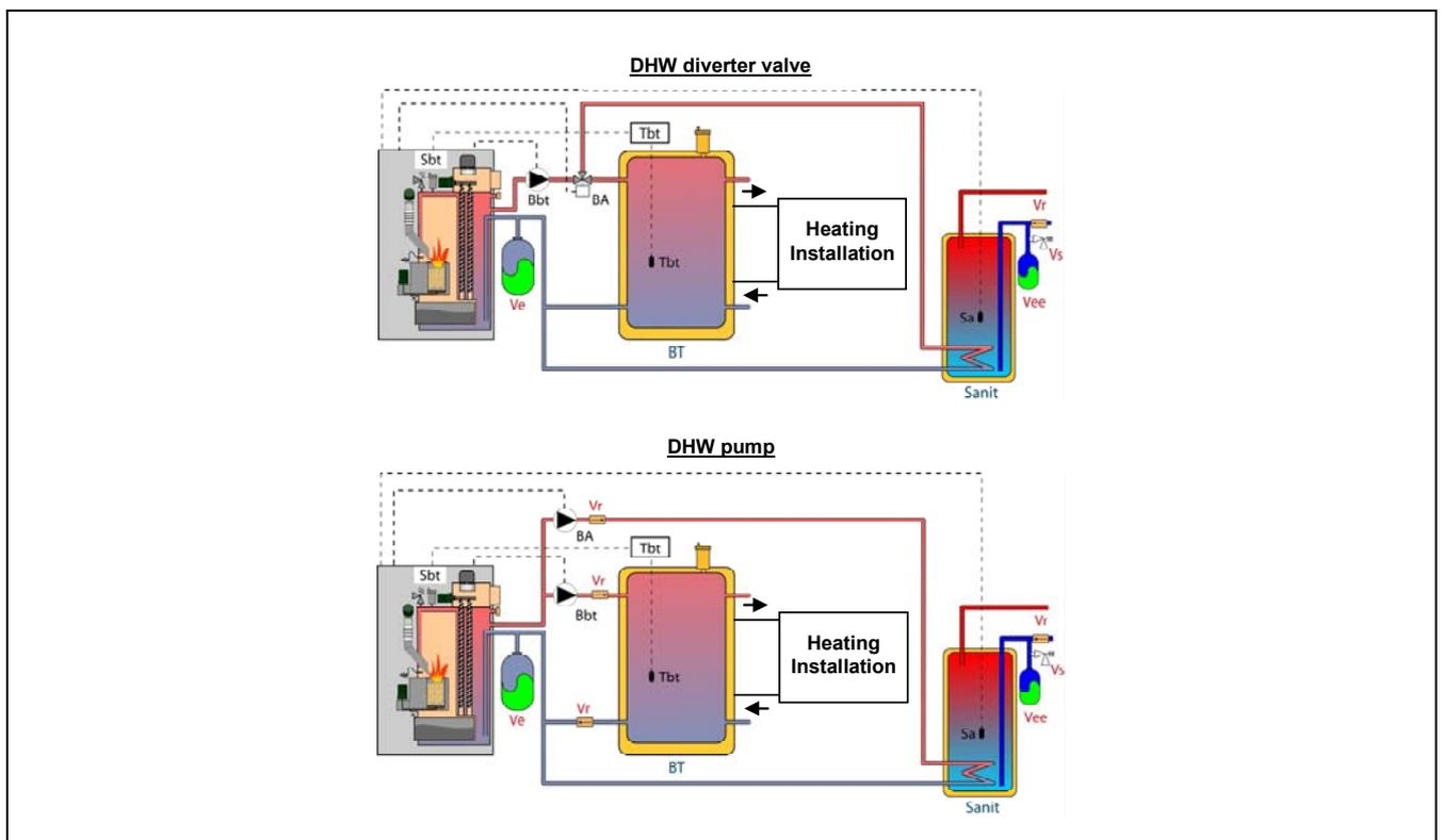
After the hydraulic installation of all the system components, proceed as follows to carry out the correct electrical connection of the BT buffer tank to the **BioClass NG** boiler:
