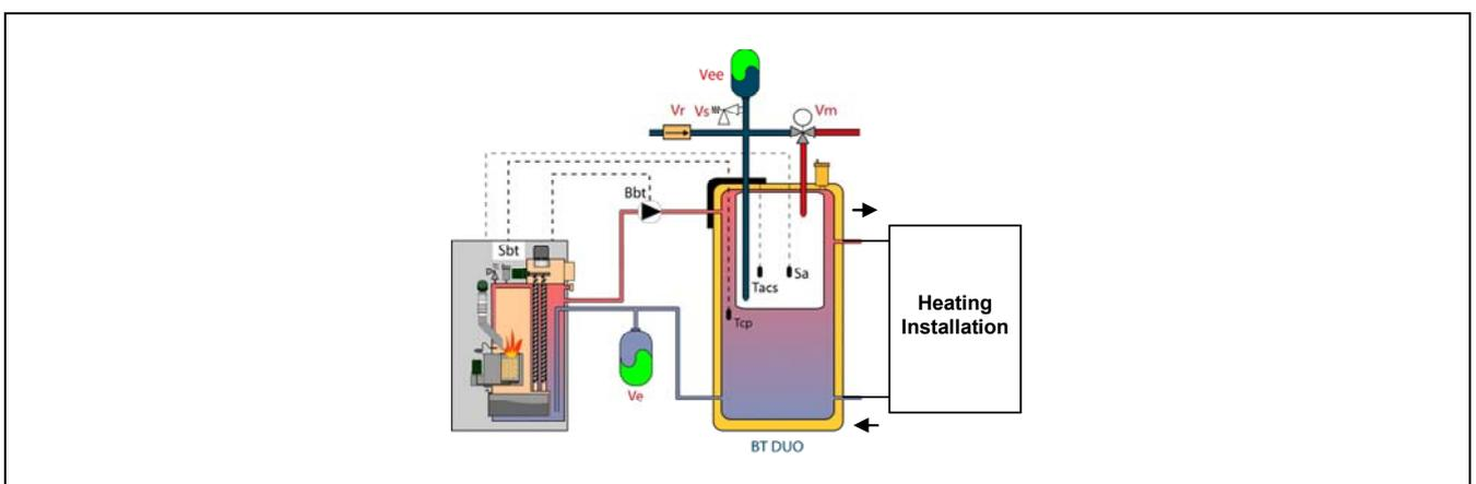
After the hydraulic installation of all the system components, proceed as follows to carry out the correct electrical connection of the BT-DUO buffer tank to the **BioClass NG** boiler:
