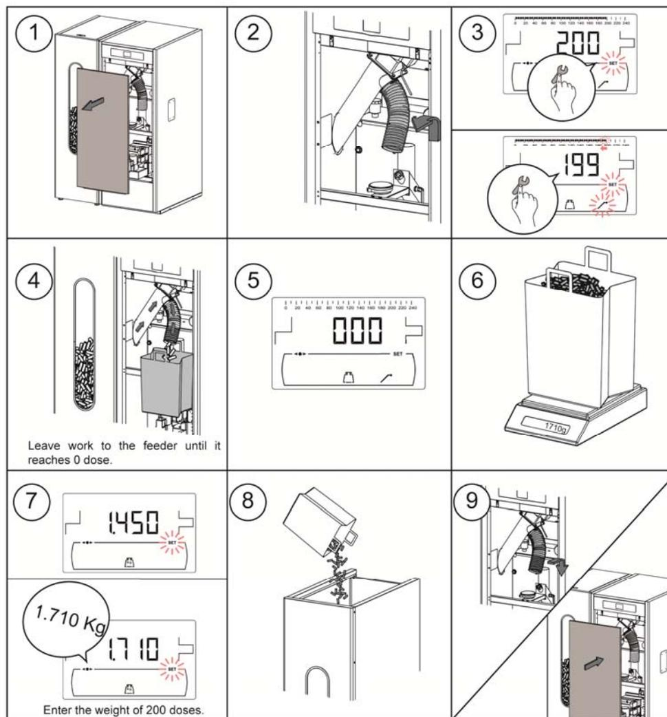
**IMPORTANT:** Calibrate the feed auger during commissioning of the boiler or whenever the fuel supplier has been changed.
