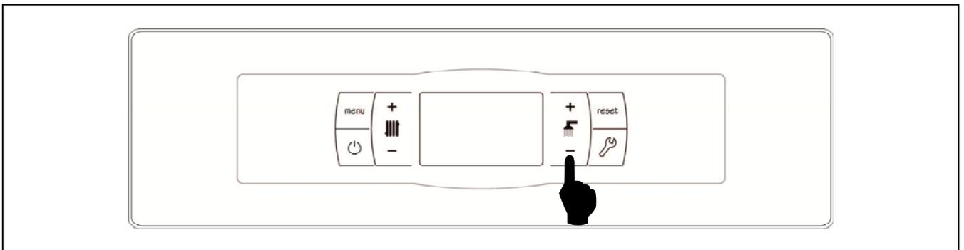
DHW temperature set point selection is made by the tactile selector shown in the picture. Press "+" and "-" buttons to increase or decrease the set point desired. Few seconds after the desired set point temperature is adjusted the display returns to main position. The range of values for DHW temperature set point is OFF, 15 - 65 °C.
