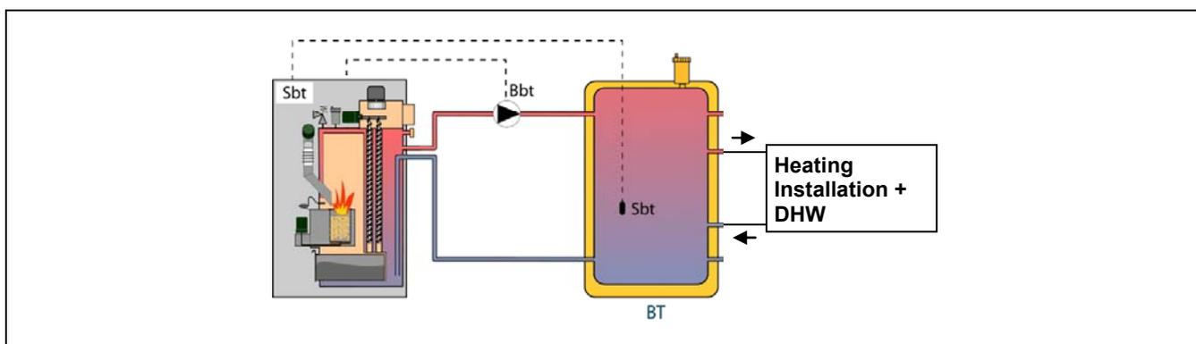
After the hydraulic installation of all the system components, proceed as follows to carry out the correct electrical connection of the BT buffer tank to the **BioClass NG** boiler:
