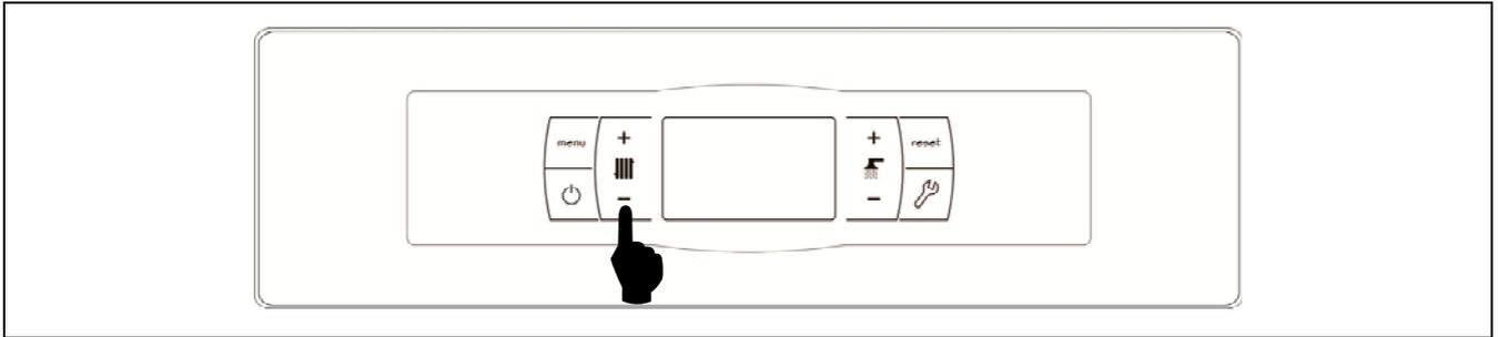
The desired buffer tank temperature is selected using the touch button, as shown in the figure. To select the desired temperature, touch the "+" or "-" symbols to increase or decrease the temperature. When the temperature has been selected, the display will return to standby mode after a few seconds. The permitted range of setpoint temperature is OFF, 30 - 80 °C.
