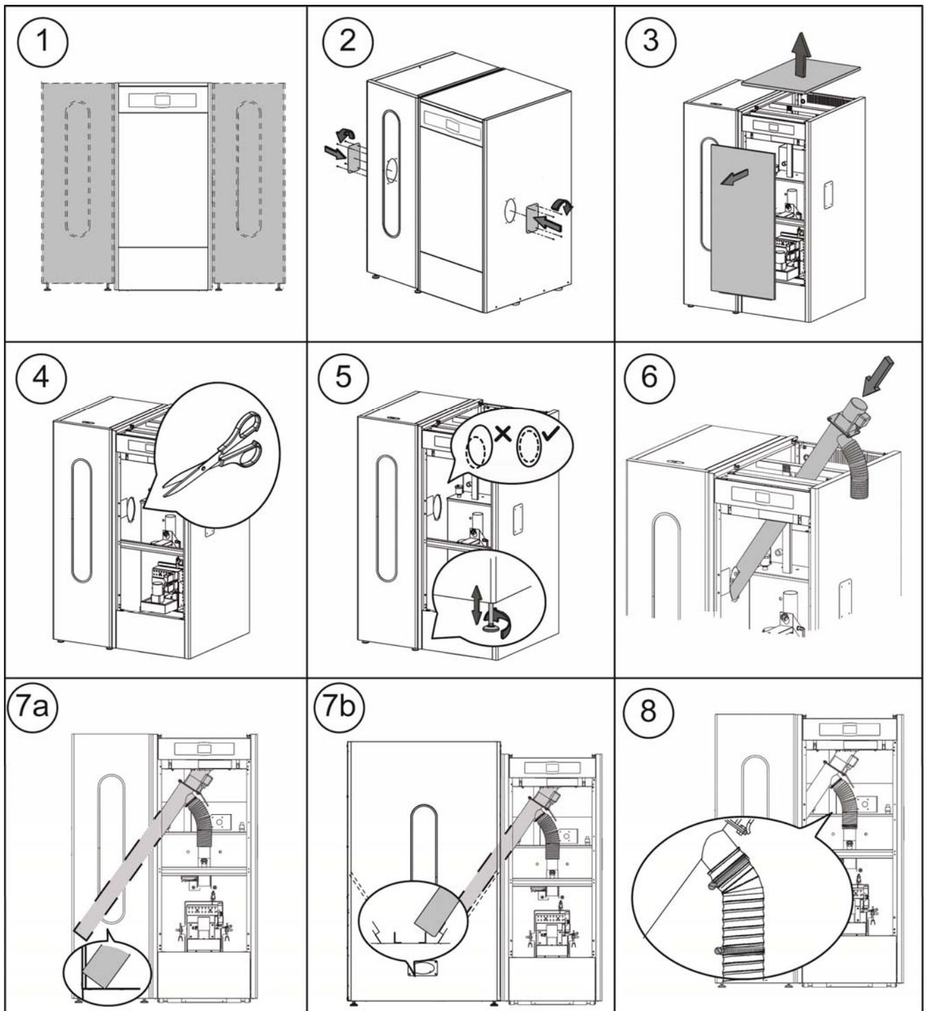
**IMPORTANT:** Ensure the height of the elliptical holes on the sides of the boiler and on the hopper coincide, for correct insertion of the feed auger. To do this, make the necessary adjustments for height (using the adjustment feet) and depth (correctly positioning the hopper).
