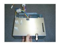
Remove the CONDENSER COVER by sliding toward.
