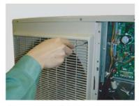
Remove the 4 mounting screws.
