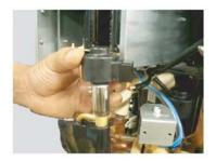
Remove the EEV coil by hand.
