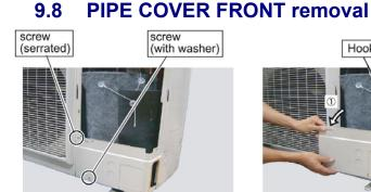
Remove the mounting screws.
