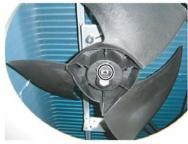
Remove the Hex Socket Screw. And remove the PROPELLER FAN.
