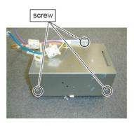
Remove the mounting screws.
