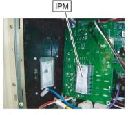
Spread the heat dissipation compound on the other side of IPM when you exchange INVERTER PCB by the repair.
