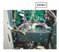
Remove the connectors, codes and screw.
