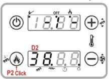
Click button **P2**: the display **D2** blinks. With other click of the button **P2** the power is changed according to the values.
