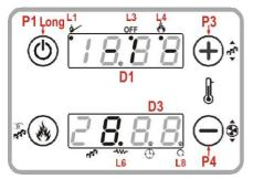
The Ignition and the Extinguishing are activated with a long pushing of the button **P1.**
