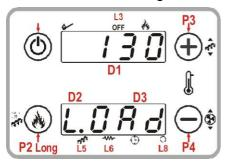
The long pressure of button **P2** activates the Pellet Manual Loading with activation of Auger engine in continuous way. The bottom display shows the actual function.
