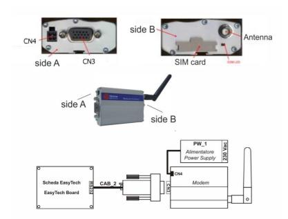
The system manages a modem module (given on demand) for the dialogue with the stove through SMS to operate the
