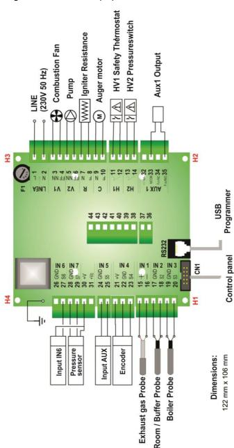
\* In case of replacing controller Version 1 (V1) with controller Version 2 (V2), wires on outputs from 1 to 14, and from 33 to 35 should be disconnect and connect again because of rotation of connecting socket!
