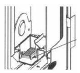
When burner apertures are filled with impurities, open and clean the burner.
