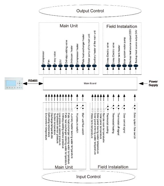
1. The environment temperature is detected by the sensor installed at fins of the finned heat exchanger, which is mainly used to control the initialization steps of the fan and the electrostatic expansion valve and also limit the maximum running frequency of the compressor. When this sensor fails, the main board will detect it and deliver this error message to the controller and then the unit will fail to start up or shut down.
