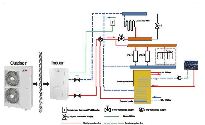
Two-way value is very important to prevent dew condensation on the floor and radiator while cooling mode.
