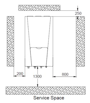
(1) Indoor unit shall be vertically mounted on the wall of the room with expansion bolt.
