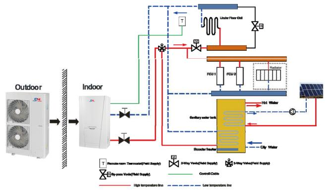
Two-way value is very important to prevent dew condensation on the floor and radiator while cooling mode.
