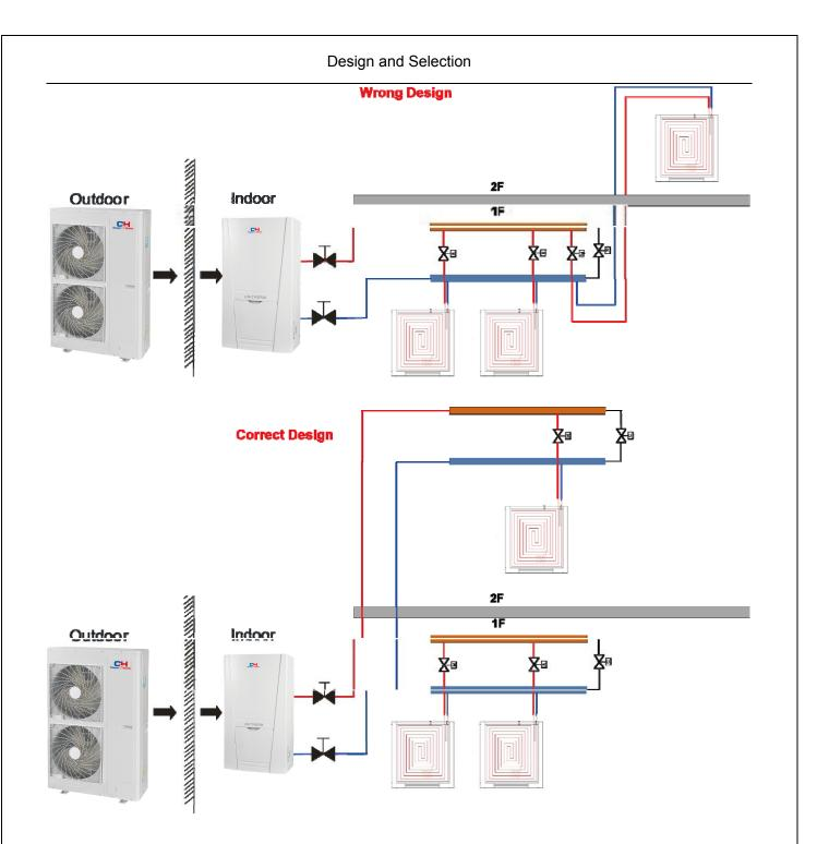
5) Distance between the unit and the water trap (collector) should be within 15m. If the distance exceeds 20m, then it is required to calculate the hydraulic power.
