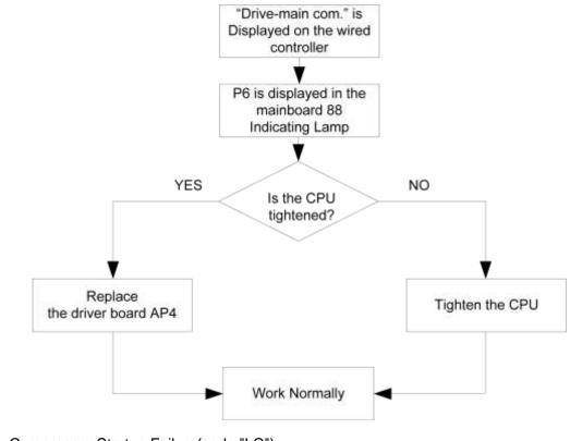
Compressor Startup Failure(code:"LC")
