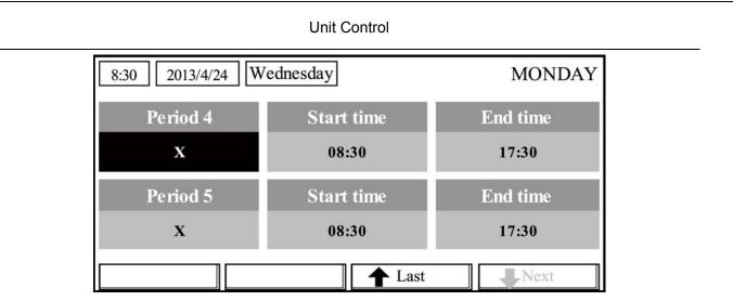
4. When above settings are finished, pressing the Return key and then pressing "**Save**", a pop-up window will pop up to remind if you are determined to save these settings. If so, press the OK key
