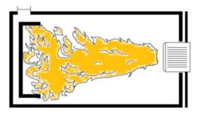
**Incorrect flame - excessive oil pressure** - remember not to overheat the furnace, as it will greatly reduce its usable lifetime. The flame must not reach the deflector. Noticing changes to the flame length, immediately change the parameters of the burner.
