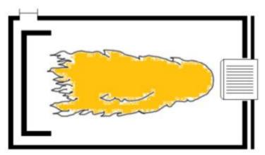
**Correct flame** - the end of the flame reaches to 2.5-5 cm (1-2 inches) before the deflector. Flame length needs to be checked periodically - initially once a week, later on once a month.
