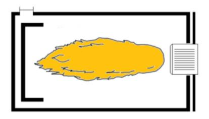
**Incorrect flame - excessive air pressure** - such a flame is equally damaging as the one above, and needs to be corrected quickly.
