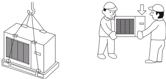
If AMS 10 must be transported across soft ground, for example a lawn, we recommend that a crane that can lift it to the set up location is used. When the AMS 10 is lifted by crane the packaging must be untouched and the load equally distributed with a boom, as illustrated above.
