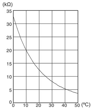
**Data for return temperature sensor (BT3), condenser supply (BT12) and fluid pipe (BT15)**
