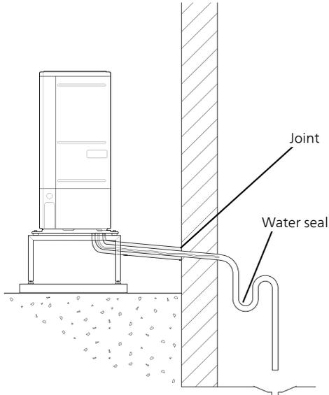
The condensation water is lead to an indoor drain (subject to local rules and regulations).
