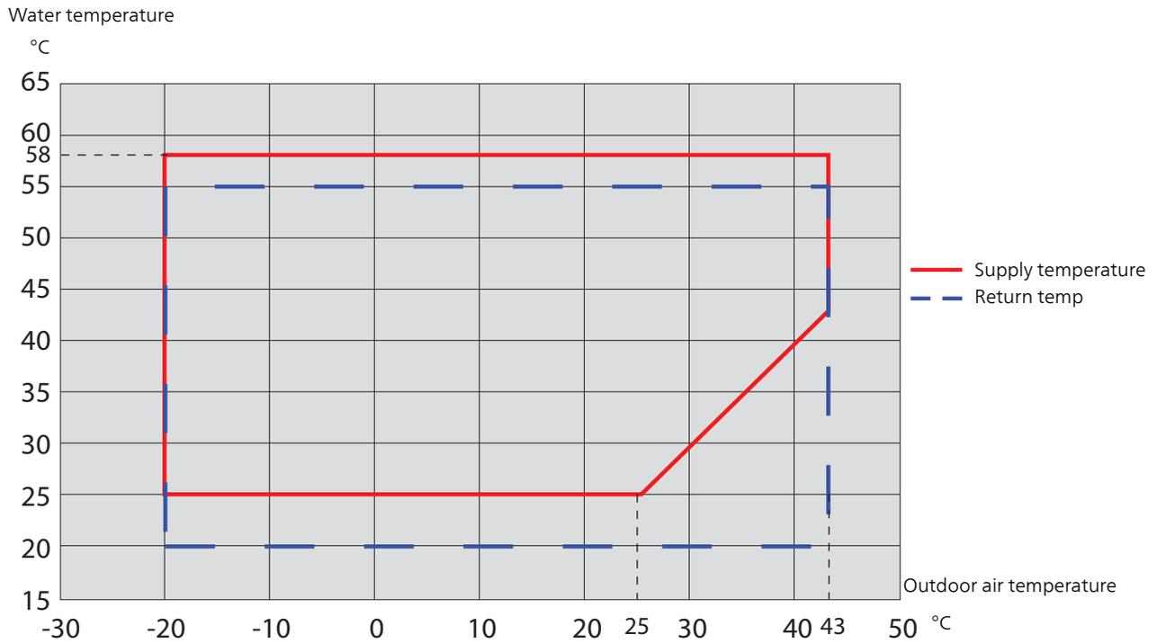
During shorter time it is allowed to have lower working temperatures on the water side, e.g. during start up.
